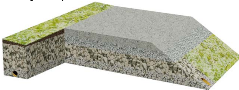
Fig. 2: Longitudinal and transverse drain (AutoCAD Civil 3D 2012).
